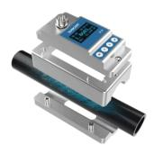
The X3 Clamp Ultrasonic Flowmeter employs the principle of time difference in ultrasonic wave propagation through the medium to precisely measure the flow rate of liquids. This advanced flowmeter is particularly well-suited for accurately gauging water consumption in residential areas, apartment buildings, and small commercial properties
