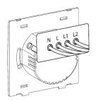
4. Fix the WS50x switch to the switch box with mounting screws, then fix the front panel back to the device.
