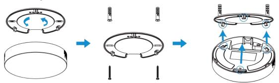
3. Align the device with the mounting plate and turn it clockwise to snap it in.
