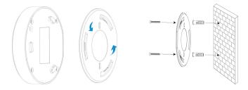
2. Turn on the device clockwise to lock it to the mounting plate. The angle of rotation can be adjusted according to your requirements (at maximum of 15°).
