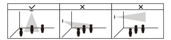
• Installation direction marking on the base, please adjust the appropriate angle according to the actual demand.
