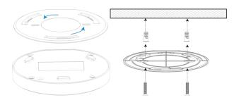
2. Turn the device clocking to lock it to the mounting plate. The angle of rotation can be adjusted according to your requirements (at maximum of 15°).
