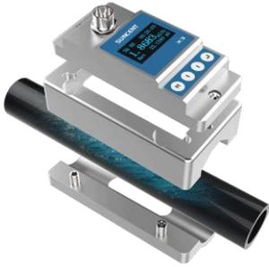
The X3 Clamp Ultrasonic Flowmeter employs the principle of time difference in ultrasonic wave propagation through the medium to precisely measure the flow rate of liquids. This advanced flowmeter is particularly well-suited for accurately gauging water consumption in residential areas, apartment buildings, and small commercial properties.
