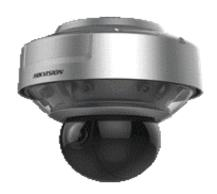
The 24-megapixel 270-degree AR spherical Hawkeye camera is equipped with 6 F1.0 large-aperture full-color lenses to achieve 270° panoramic picture stitching. It can be widely used in urban high points, airport terminals, construction sites, industrial parks, and other locations.
